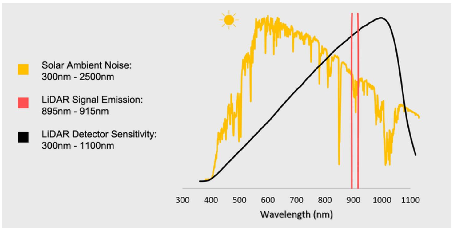
Application of Visible Opaque materials formulated with specific NIR absorbers effectively filters both visual and NIR noise that lies outside of the targeted LiDAR signal band. Such light management techniques can dramatically improve LiDAR resolution and range.
